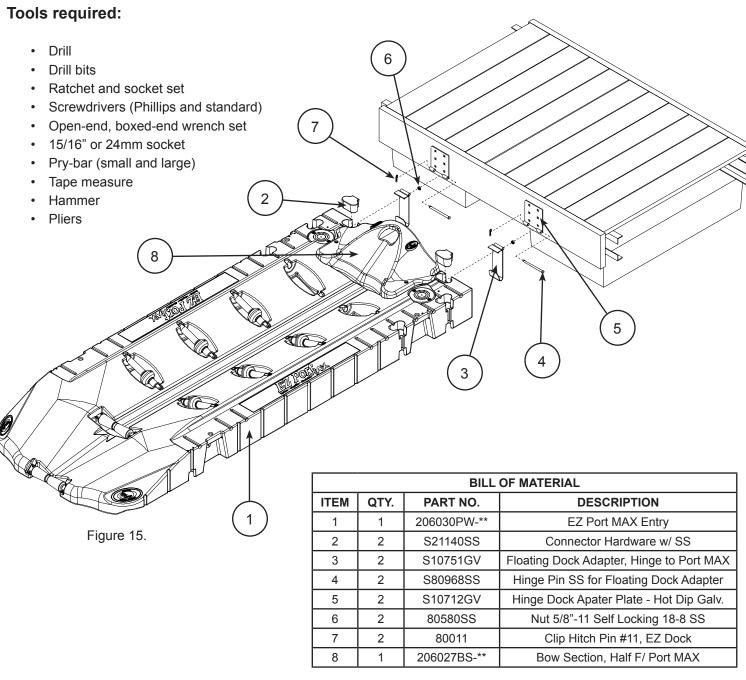
The hinge dock adapter plate, (Item 5), may be installed with the hinge point on the top as shown, (Figure 16). All other installation is the same as on previous page.
