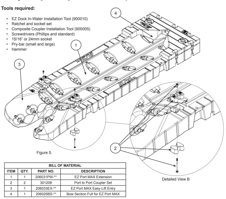
**NOTE:** Testing has also shown that some watercrafts and user preference resulted to water ballasting the entry (206033EX-\*\*) with water (see EZ Launch Owners Manual). This is done by simply filling the entry with water to the desire level. This allows the watercraft an easier entry and even a more stable platform.
