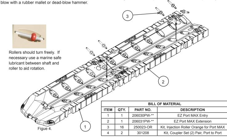
**Step 3:** Assemble a Full Bow Section at the front of the EZ Port MAX Extension. (See page 8, Figure 2 for Full Bow Section assembly instructions).
