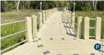
POLY POST HANDRAILS Attaches to the coupler pocket. Can be used as a grab or accessory attachment post. 8 embedded T-nuts for cleat attachment, and recessed holes that can be drilled for tube or rope handrails. (Handrails and Cleats not included.)
