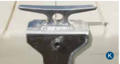
TIE-DOWN CLEAT Tie-down cleat (10") and other accessories attach to heavy-duty stainless-steel T-nuts molded in pairs around dock section perimeters.
